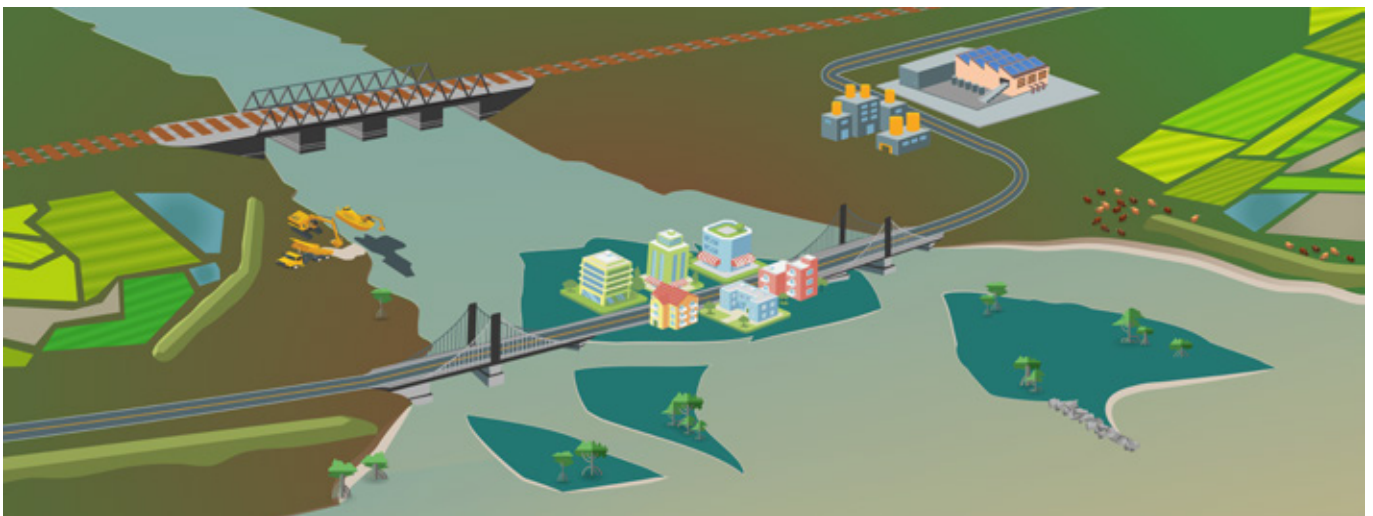
Fig 5b.i: Deltas after human impact: the natural equilibrium is disturbed. Sediment replenishment decreases due to dams and sand mining. Sediment movement and deposition in floodplains are affected by levees, embankments, roads and railways. Sediment replenishment further decreases due to dikes and polders.
